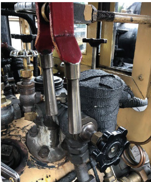
Turret with atomising steam valve and steam separator.
