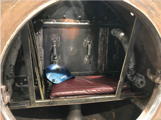
NG/G16 Spark arrestor fabrication
